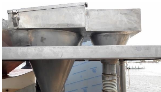
Figure 2: Dual entry feed to discharge prawns onto the stunner conveyor.
